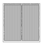
Figure 21 - Correct Burner Flame Pattern
